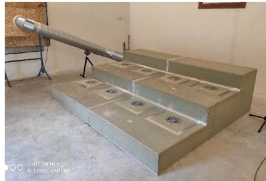
Figure 2 Model of bleachers with 8 diffusers
