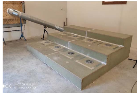
Figure 2 Model of bleachers with 8 diffusers
